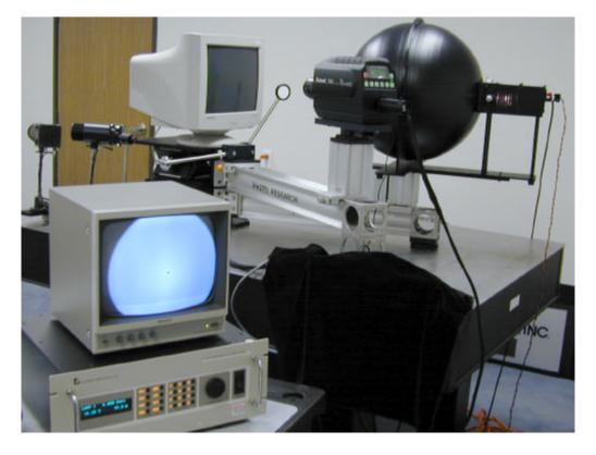
PR<sup>®</sup>-P7 System for ISO 9241-7 Reflection Measurements
